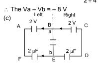
From the figure it is cleared that the left and right branch are symmetry and reversed, so the current go towards BE from BAFEB same as the current from EDCBE.
