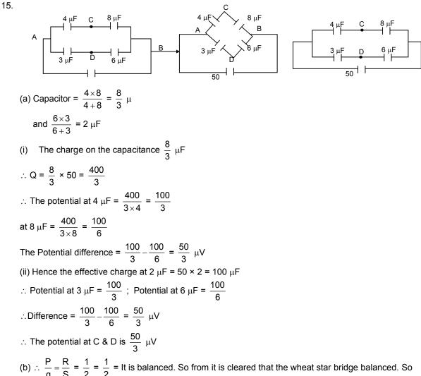
the potential at the point C & D are same. So no current flow through the point C & D. So if we connect
