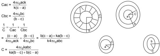
62. These three metallic hollow spheres form two spherical capacitors, which are connected in series. Solving them individually, for (1) and (2)
